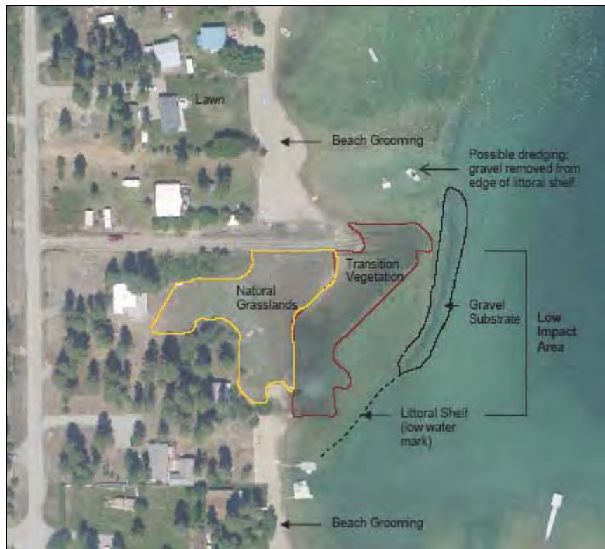
Figure 23. Overview of properties along Segment W3, showing area where the natural shoreline features were kept intact (low impact area) against adjacent properties where development has substantively altered the shoreline.
